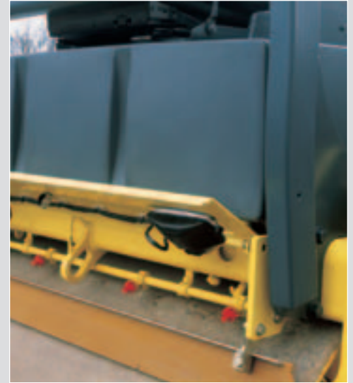
Wind protected spray nozzles for even drum coverage
