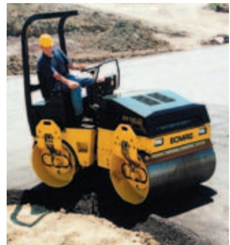
BW135AD in action on asphalt
